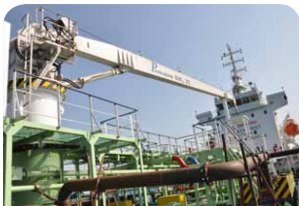
Cargo Hose Handling Crane
